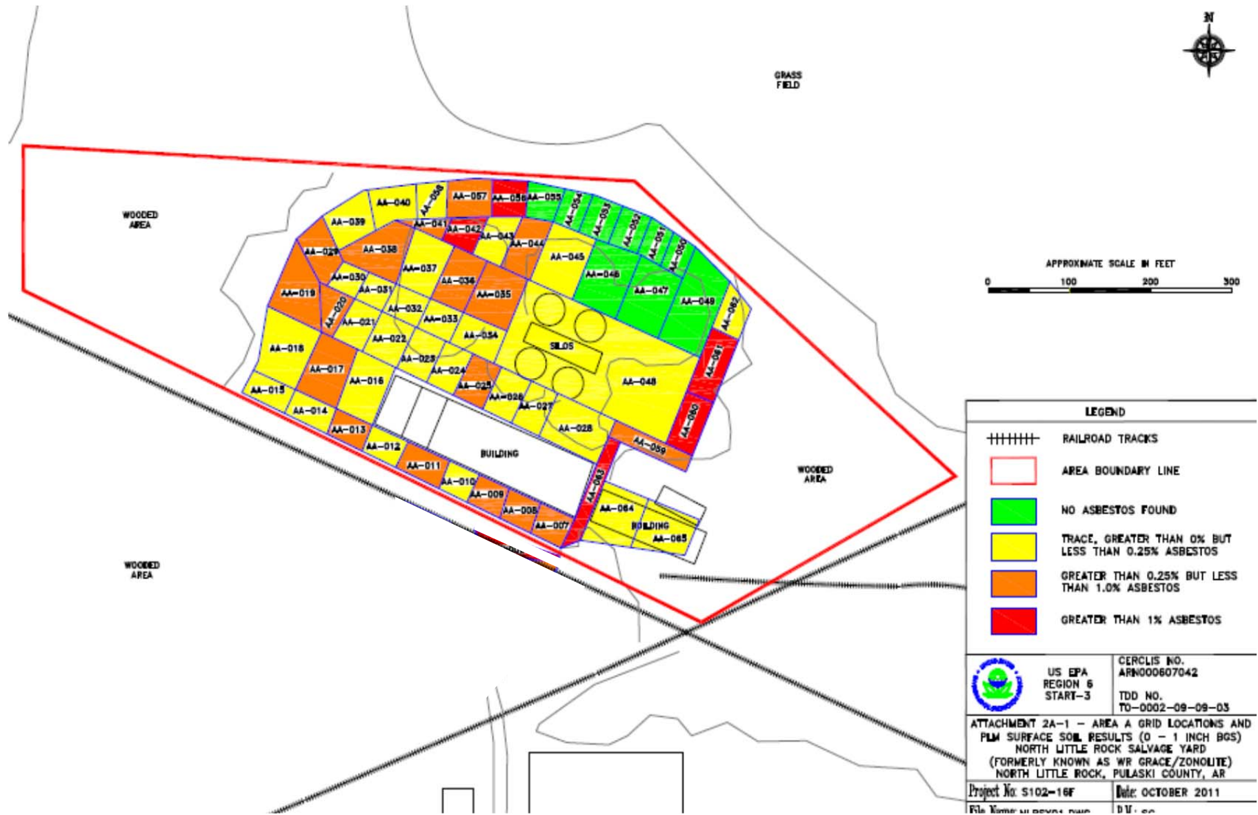
Figure 2. Grid Layout for EPA Soil Sample Collections (0 – 1 inch) at the Former W.R. Grace Facility
