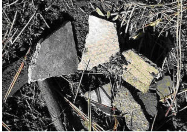
Figure 6: Cement Asbestos Board
