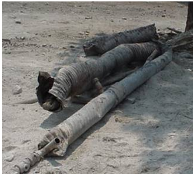
Figure 9: Asbestos-Containing Steam Pipe
